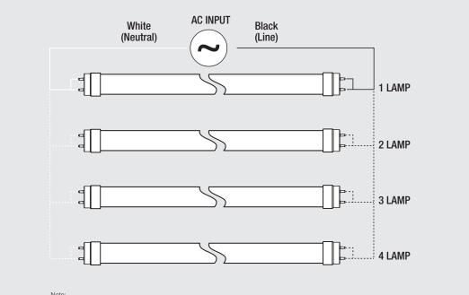
Note: 1. LEDIescent" lamp is polarity neutral. Can be installed in either direction. 2. Sockets may be shunted or non-shunted. Tie socket leads together for non-shunted sockets.
