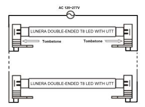
Note: Add jumper wires to shunt the tombstones or connect hot and neutral pins marked L and N.
